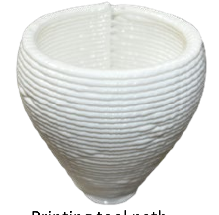
Printing tool path demonstrated on “miniWAAM”
