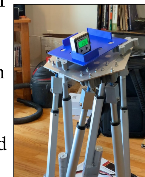
Rotation range measured with a digital angle meter
