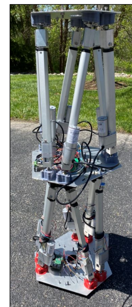
Two Stewart platforms stacked on top of each other
