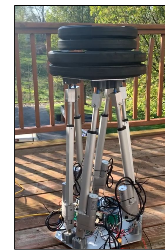
Lifting force exceeds 140 lbs in pure vertical movement
